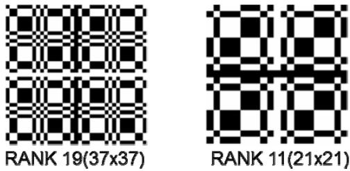
Fig. 1. Simulated collimator pattern (MURA).
